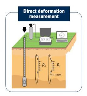
Also refer to our Data Sheets on the Medusa DMT and Seismic DMT for full details of our DMT testing capability.
