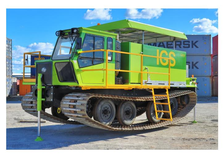
Purpose-built rig on Prinoth Panther Base Year Built: 2020 High Accuracy GNSS GPS on board Mass ~16t W=3.03m L=7.4m H=3.01m (roof down) Push capability 150kN Variable Push Speed from 20mm/s to 200mm/sec Movable Pusher – can do two test/sample pushes at one set-up Very wide tracks giving approx. 20kPa ground pressure Rear mounted winch, 16mm dyneema, 27t MBS – 70m length AS1657 compliant access and egress Built to satisfy mine regulations
