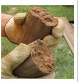
Our Vertek Ranger Samplers are floating piston devices that can take samples in almost any soil type. Diameters: 35mm, 46mm, 66mm. Samples can be tubed or bagged.
