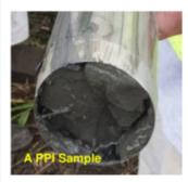
Our flagship sampler. This takes 63 or 75mm diameter samples about 800mm long that are arguably as close to undisturbed as you can get by any means other than research-level block sampling.
