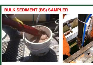
Our BS Sampler is used to air lift "ooze-like" samples (eg semi-liquid tailings) from any specific depth. Very large bulk samples can be taken, that are not water-diluted.
