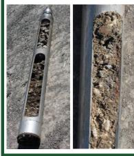
Window Samplers can be used to (a) take samples of coarse and gravelly material (eg rail ballast and subgrade), or (b) to pre-core through a stiff surface layer to allow other testing and sampling below. Telescoping design,
