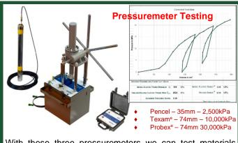
With these three pressuremeters we can test materials ranging from soft clays to medium strength rock, in boreholes and (with the Pencel) also by direct-push.
