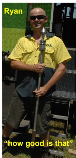
63mm 316 stainless sampler with 1.6mm wall thickness. An 800mm long sample is taken using the "stationary piston" technique. Sample quality is enhanced markedly by direct air injection at the cutting face to cut the sample free and then injection is continued to eliminate suction during extraction.
