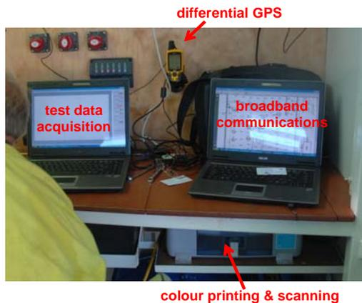
Each IGS rig has full-time on-board broadband connection independent of its data acquisition system. Also colour printing and differential GPS.
